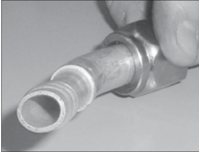
Incorrect tube and hose combination causing tube to seriously deform.
