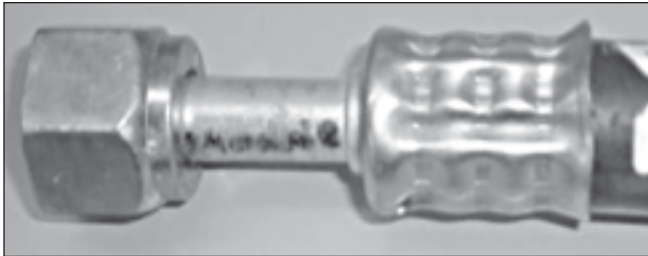
Assembly crimped, rotated and re-crimped.
