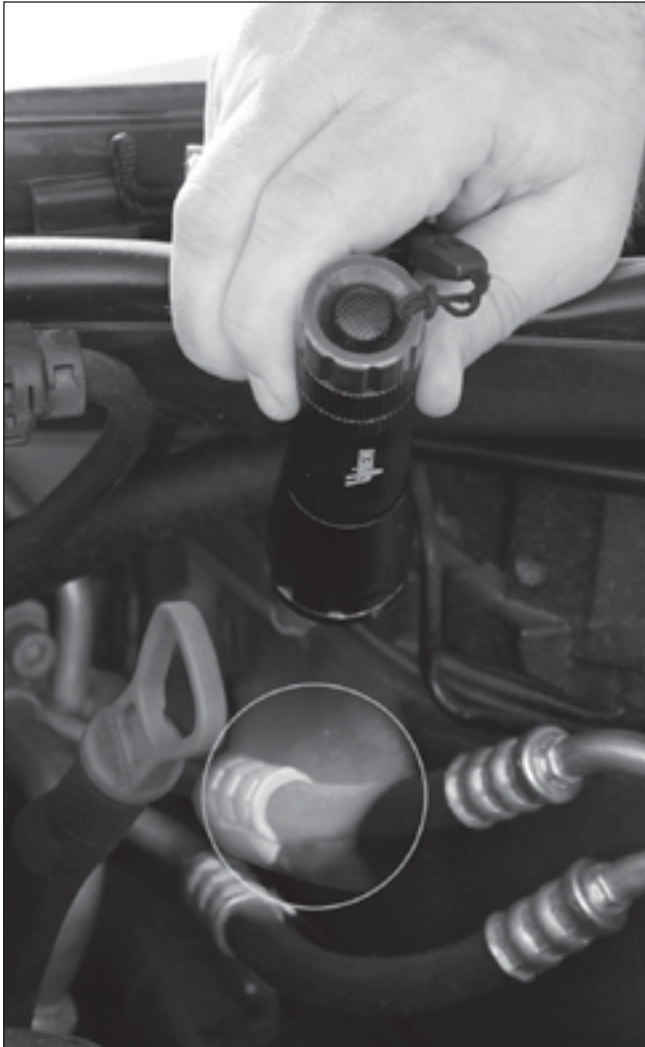
The leaking dye will glow under ultraviolet light. (Courtesy CPS Automotive Group)
