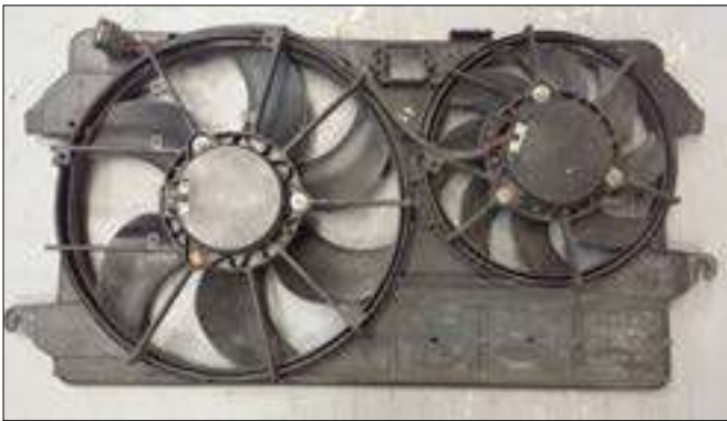
Figure 2: The electric cooling fans on modern engines are usually controlled by the PCM (powertrain control module).
