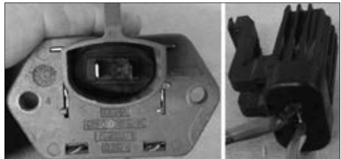
Figure 6: Burned cooling fan resistor and connector from a 2011 Ford Transit Connect
