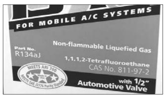
Make sure new HFC-134a you intend to purchase meets the SAE J2776 and/or the ARI 700-2006 purity standard(s), and has a 1/2-inch Acme tank fitting.
