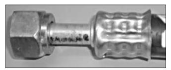
Assembly crimped, rotated and recrimped.
