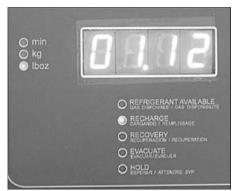
This machine is displaying the refrigerant charge amount in pounds and ounces. However, the label on every vehicle you service won't list the spec this way, so calculations will be needed; an easy place to make a mistake. (Some machines allow you to change the display units, but how many techs do so every time they can or should?).
