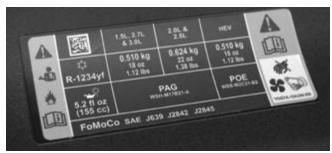
A vehicle's A/C system information label lists the type of lubricating oil that the system requires.
