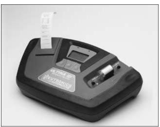
While not required by federal law, the use of a refrigerant identifier is strongly recommended. It can help you determine if a vehicle contains contaminated refrigerant that you would not want inside your recovery machine. Identifiers can also provide an accurate indication concerning the amount of air that may be in an A/C system or storage tank. Some state or local laws may require their use.
