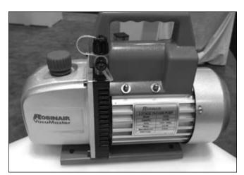
To assure proper performance, vacuum pumps must be serviced at the intervals specified by their manufacturers. Vacuum pump service usually consists of not much more than changing the vacuum pump's oil. Typical vacuum pump oil change intervals run from the oil needing to be changed after every 10 hours of pump operation. Consult your vacuum pump's operational manual to find out how often you need to change its oil.
