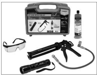
A typical UV dye leak detection kit contains dye, a dye injector (or some other type of tool to introduce dye to a system), a UV flashlight, and the correct goggles for the dye being used. Always wear the goggles to protect your eyes from the UV light. This kit also contains a special cleaner to remove traces of the dye after the leak is repaired.
