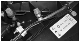
The caps are the service ports' primary seal against refrigerant leakage. Always make sure that every service port has one in place.
