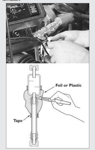
To help confirm a suspected leak, place aluminum foil or plastic wrap and tape it around the connection or component. If there truly is a leak, after a few minutes, refrigerant should accumulate inside the plastic wrap or foil. Make a small hole in the foil or wrap at the lowest point possible and place your leak detector probe at the hole. The detector will indicate "refrigerant found" if a leak is actually present.
