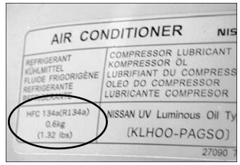
Infiniti (M45) label shows refrigerant capacity in pounds and kilograms, but with no tolerance listed.
