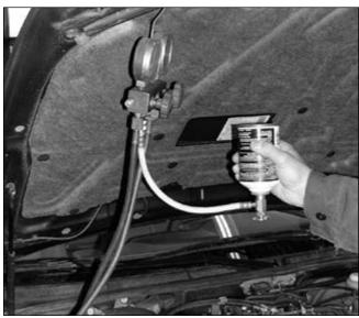
Some technicians still attempt to use small cans and pressure gauge readings to charge systems, but accurate charging is not possible with this method.
