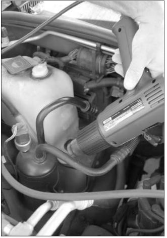
Heating an accumulator during refrigerant recovery is a good idea. The heat will raise pressure inside the accumulator, allowing it to more easily outgas refrigerant it contains. This will reduce the amount of time necessary for more complete refrigerant removal.
