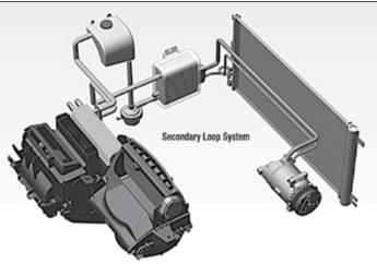
Most A/C systems are Direct Expansion, meaning the refrigerant directly expands within the evaporator that's located inside the passenger compartment. For safety reasons, systems designed to use R-152a will be Secondary Loop, instead using a refrigerant-to-glycol heat exchanger located inside the engine compartment. Chilled glycol will then circulate through a Cooler Core of sorts, to remove heat from the cabin.
