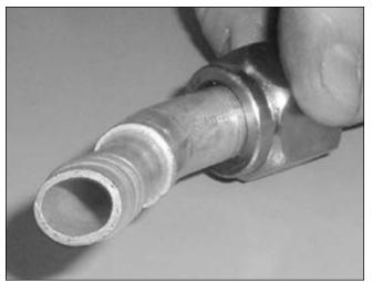
Incorrect tube and hose combination causing tube to seriously deform.
