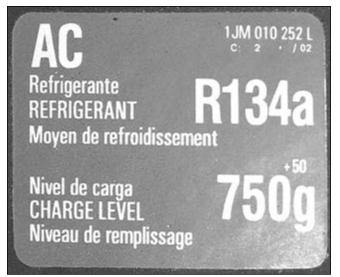
This Volkswagen label gives refrigerant capacity in grams, along with the plus tolerance (notice there's no minus, so the range is 750-800). In this case (although ounces are not listed), the specification tolerance of 50 grams can be rounded off to two ounces in any conversion.
