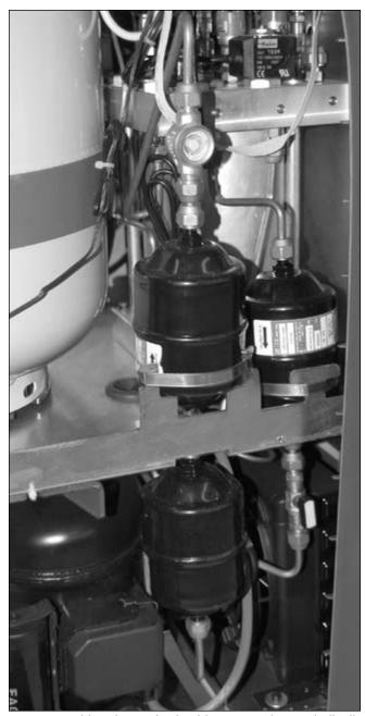
R/R/R machine internal plumbing must be periodically checked to make sure no leaks are present.
