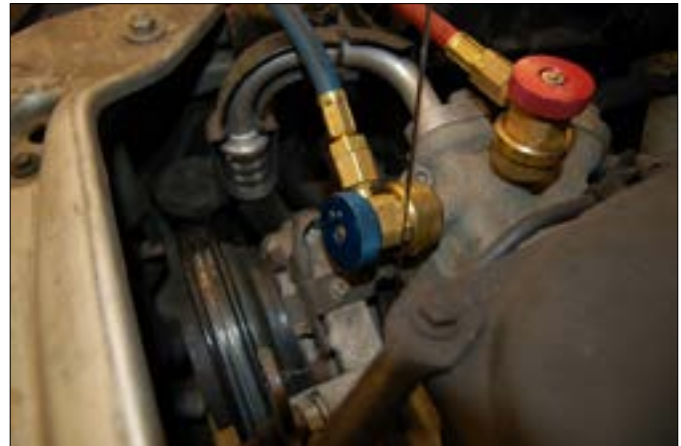
Figure 1: Having the service ports located right at the compressor, such as on this manifold, ensures being able to get the actual pressures the compressor is producing (unless there is a problem with a Schrader valve, hose connector, gauge or hose connected to the gauge).
