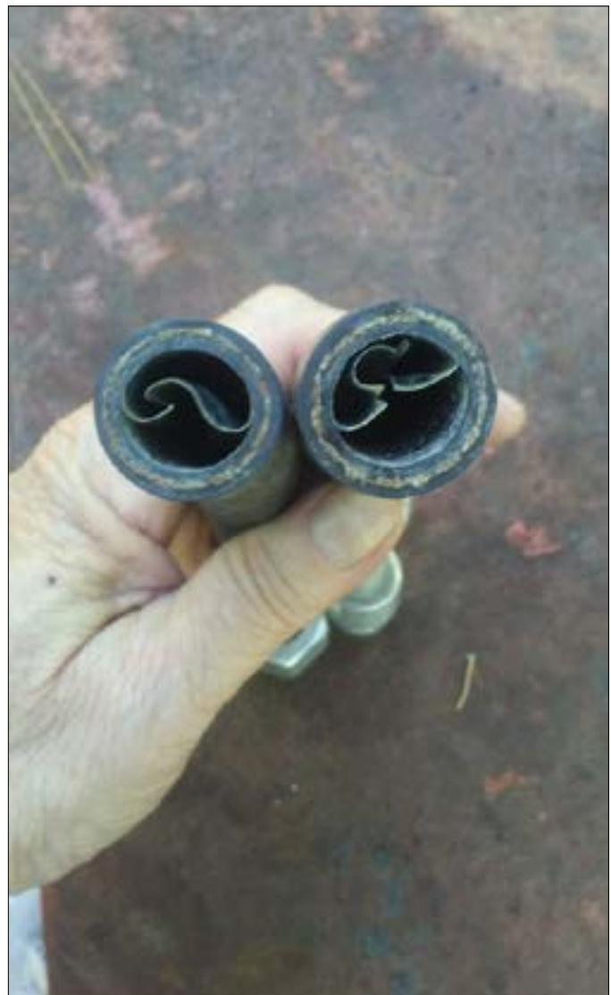
Figure 9: Cutting the hose in two at about the midway point revealed exactly what the problem was. The inner liner had come loose from the adjacent layer it had been attached to.
