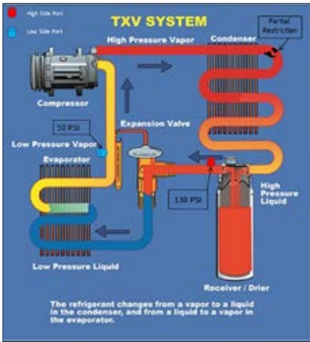
Figure 5: Expansion Valve System with a restricted condenser.
