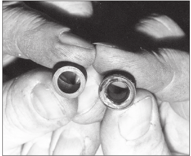
The seals on service equipment hoses must be frequently inspected for damage and replaced when necessary. This shows a comparison between a new seal (left) and a used one that is swollen and distorted (right).
