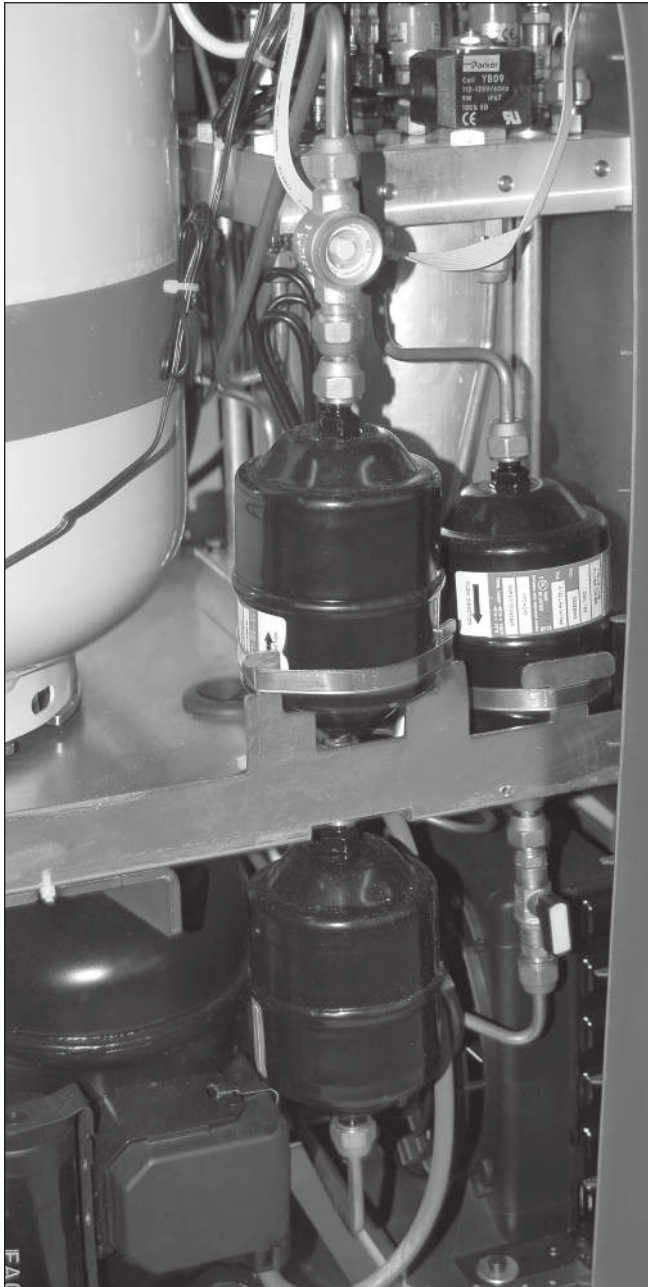
R/R/R machine internal plumbing must be periodically checked to make sure no leaks are present.
