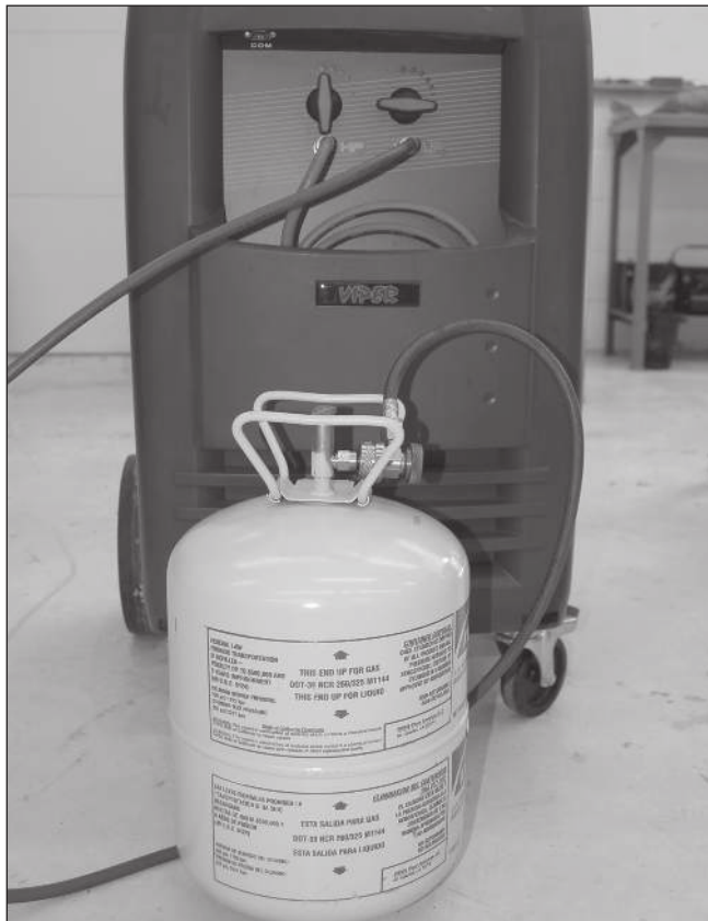
Before they are discarded, disposable refrigerant cylinders should be connected to recovery equipment and brought to a vacuum. This will ensure that all refrigerant has been removed.
