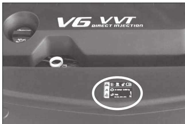
The refrigerant label is easy to find on the 2013 Cadillac XTS but you may have to look around on other vehicles.
