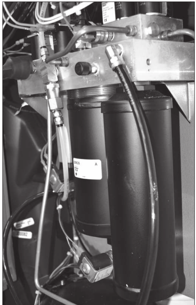
R/R/R machine filters/driers must be replaced in accordance with the machine manufacturer's recommendations.
