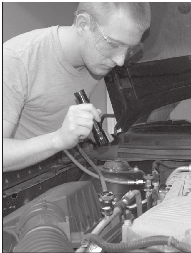
Like this technician, always be sure to wear the special goggles that came with your UV dye leak detection kit. Not only do they protect your eyes from the UV light, they also make dye traces at leak sites stand out better.
