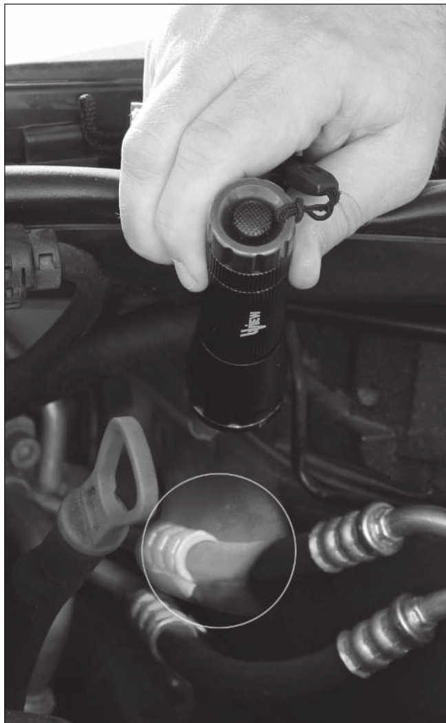
The leaking dye will glow under ultraviolet light.
